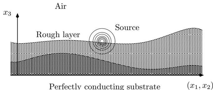
FIGURE 1.1. *Setting for the rough layer scattering problem. Points in  $\mathbb{R}^3$  are denoted as  $x = (x_1, x_2, x_3)^\top$ . The penetrable layer has finite distance to the hyperplane  $\{x_3 = 0\}$ . We seek the wave field due to a time-harmonic source situated in a neighborhood of the layer.*
