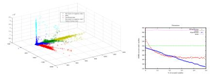
Fig. 1.3 (a) Automatic segmentation of Highway data projected on 3-d dominant PCA space. (b) Error on travel time for a BP prediction of 3 time layers in future as a function of the fraction of observed variables at  $t_0$ . Comparison is made with a predictor combining recent available observations with historical time dependent mean.
