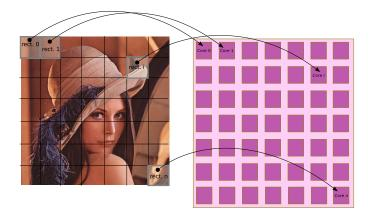
Fig. 6. Scheme of affectation of source image parts to each core in our benchmark program
