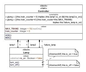
Figure 2: Block definition diagram of the case study SysML model
