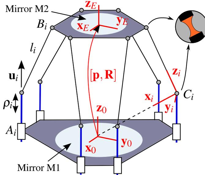
Figure 2: Kinematic structure of the space telescope
