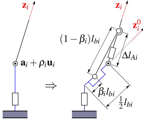
Figure 10: Kinematic model of a flexure joint
