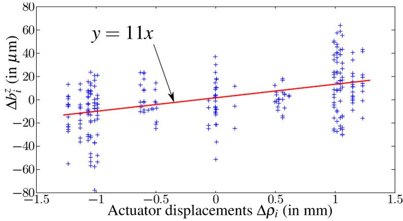
Figure 7: Linear approximation of the platform deformation
