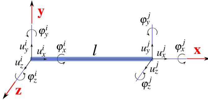
Figure 11: Local coordinate system of a flexure joint
