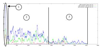
Fig. 3. PER evolution (%) vs time (s) over the first hour for each link (Red: pelvis, Green: left foot, Blue: right foot); 3 phases: 1. Beginning of the race, difficult contact; 2. High density evolution; 3. Lower density, quasi-LOS transmission.
