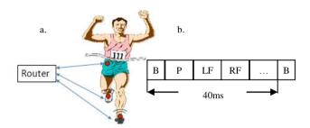
Fig. 2. a: Star network configuration. b: Periodical TDMA protocol (4 emission slots, B: Beacon, P: Pelvis, LF: Left Foot, RF: Right Foot, remaining time used for the data acquisition).
