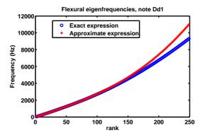
(b) Low frequency behavior of the flexural branch  $f_{\ell}^{-}$  of equation (17) (in blue) compared to its approximate expression for small  $\ell$  of equation (19) (in red).
