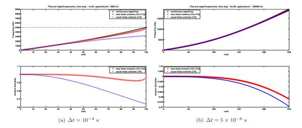
FIGURE 5 – Comparison of theoretical eigenfrequencies of the continuous system (black circles  $\circ$ ), new  $(\theta, \overline{\theta})$ -scheme with  $\theta = 1/4$  and  $\overline{\theta} = 1/12$  (red dimonds  $\diamond$ ) and usual  $\theta$ -scheme with  $\theta = 1/4$  (blue plus sign +). The theoretical curves are plotted for the first eigenfrequencies after which numerical stability is no longer granted.
