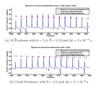
FIGURE 4 – Transversal displacement's spectrum of string D $\sharp$ 1. It is clear that the new  $(\theta, \overline{\theta})$  reduces numerical dispersion from the continuous eigenfrequencies, compared to the usual  $\theta$ -scheme, with no computational overcost.
