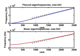
(a) Two branches of eigenfrequencies : upper figure (in blue) for flexural frequencies  $f_\ell^-$ , lower figure (in red) for shear frequencies  $f_\ell^+$ . The high frequency behaviors are represented in dashed lines.
