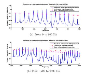
FIGURE 3 – Transversal displacement's spectrum of string D $\sharp$ 1 using a  $(\theta, \overline{\theta})$ -scheme with  $\theta = 1/2$ ,  $\overline{\theta} = 1/4$  and  $\Delta t = 10^{-4}$ .
