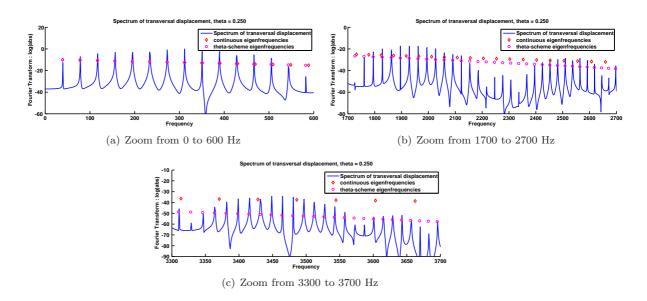
FIGURE 2 – Transversal displacement's spectrum of string D $\sharp$ 1 using a  $\theta$ -scheme with  $\theta = 1/4$  and  $\Delta t = 10^{-4}$  s.
