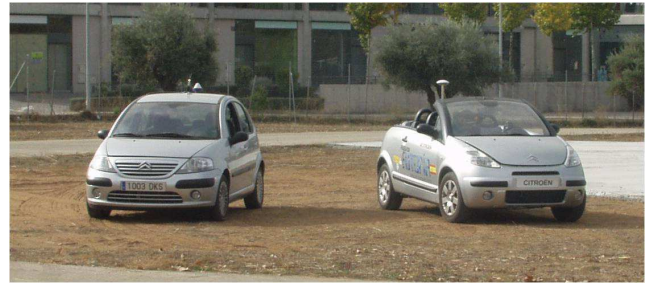
Fig. 3. Convertible Citroen C3 Pluriel fully automated and Citroen C3.
