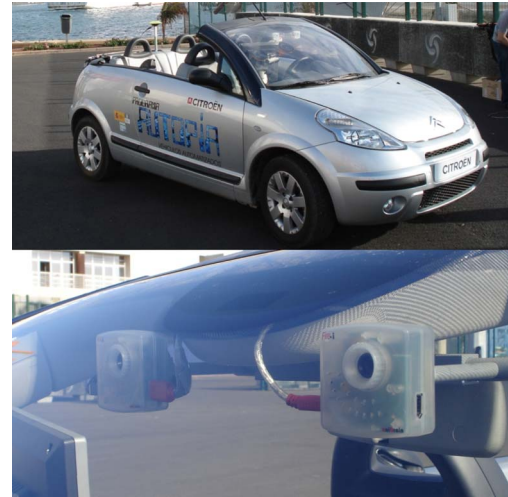
Fig. 1. Experimental vehicle and the onboard stereo sensor.
