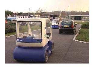
Figure 7. Co-operative overtaking maneuver through co-operation with vehicles driven by human beings [27]
