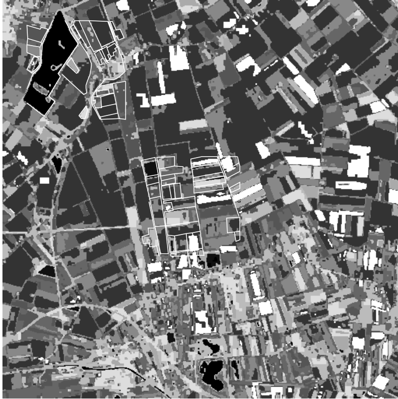
Fig. 3.21 Hierarchical segmentation result with 10 classes (ICM).
