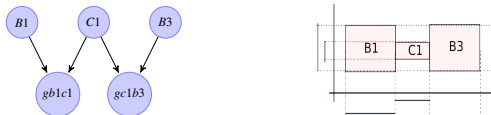
Figure 22: In the left, the adjacency relation is presented by hierarchical relation and in the right, by topological one.
