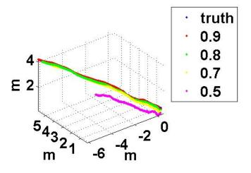
Figure 7: Trajectories estimated by the EKF when the state is initialized with an absolute scale which is smaller than the true one (in particular, up to half time the true value).
