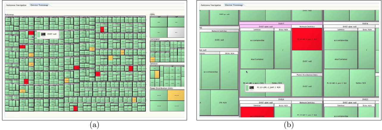
Figure 6. (a) Synthesized view of hardware devices as a treemap, for monitoring purposes. (b) Zoomed-in view focusing on a particular device and its sub-hierarchy, that features a faulty component (colored red).
