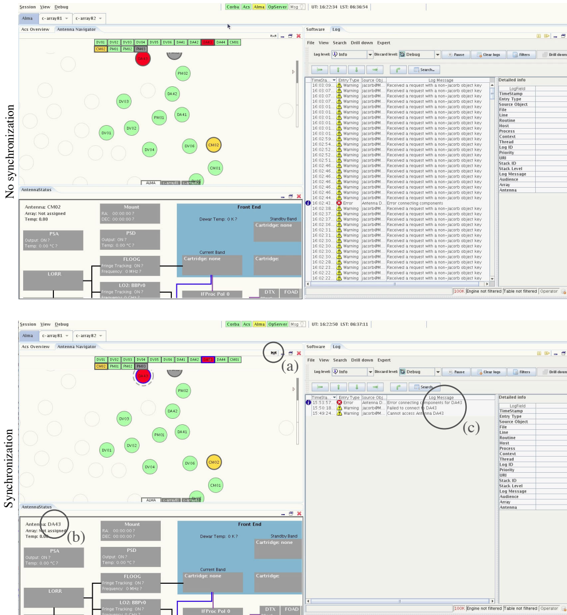
Figure 8. Top: Three independent user interface components that give complementary views of the system. Bottom: the antenna map can be coordinated (a) with both the AntennaStatus panel and the logging panel (a). Then, whenever the user selects an antenna in the chessboard or the map (here DA43), the AntennaStatus panel gets automatically updated to show DA43's block diagram (b), and the logs get filtered to only show entries related to that antenna (c).
