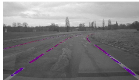
Fig. 3: Road marking feature extraction
