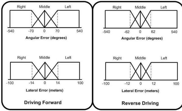
Fig. 4. Membership functions of the lateral fuzzy control.
