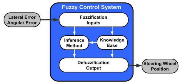
Fig. 3. Fuzzy control system of the steering wheel.
