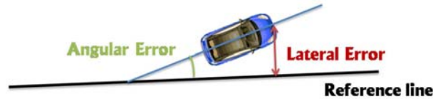
FIGURE 3. Graphical representation of the input variables (lateral and angular error) with respect to the reference line
