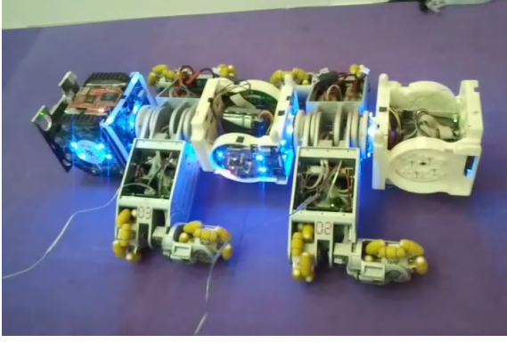
Figure 1: Five modules connected together to form a larger organism in the Symbion project. Each module embeds its own controller and communicates with its neighbors.
