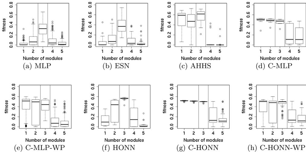
**Figure 8: Generalization capability of the best controllers evolved for three carts, in the multipole-no-velocity benchmark. Each controller is re-evaluated with 1, 2, 4, and 5 carts to assert its transferability in a different setup. Neat and HyperNeat are omitted due to poor performance (similar to MLP and ESN).**
