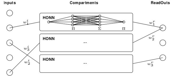
**Figure 4: Structural description of a C-HONN. A C-MLP is described in a similar fashion by replacing the embedded HONN networks by MLP networks with one hidden layer. Similarly, C-HONN-WP, resp. C-MLP-WP, accept the same description, with embedded HONN, resp. MLP, as copies of a specific reference template (i.e. an evolved pattern).**
