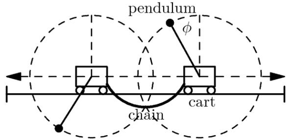
**Figure 3: Coupled inverted pendulum benchmark with two carts, pendulums are free to move full  $360^\circ$  mounted on the carts that move in one dimension (left/right) bounded by walls (track ends) and other carts. Marked angle is pendulum angle  $\phi$ .**
