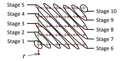
Figure 4: The origin of the data in input of the North port of a router r stages after stages.
