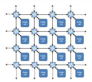
Figure 1: A 2-dimensional CA with bidirectional channels.
