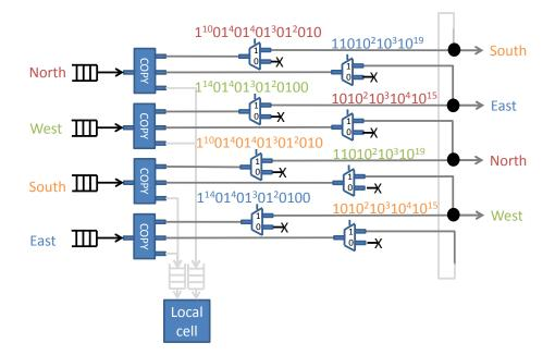
Figure 5: The internal crossbar of the router with the switching conditions.
