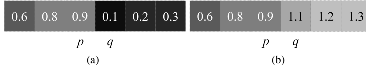
Fig. 2.4 One-dimensional phase unwrapping example. (a) Measured phase image. (b) Unwrapped phase image where the phase difference between p and q is now less than 0.5 . In (a) and (b), all the phase values have been divided by 2\pi . For example, the displayed value 0.1 corresponds to 0.2\pi .
