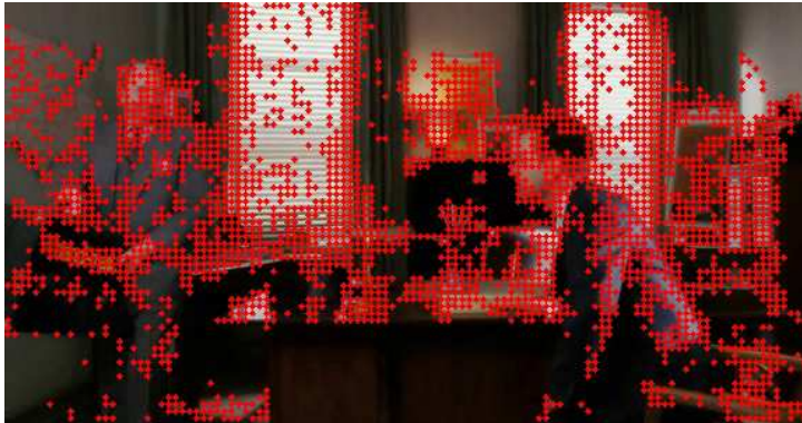
Figure 3: Visualization of densely sampled feature points after removing points in homogeneous areas using the criterion in Eq. (1). We only show feature points in the first spatial scale. The sampling step size W is 5 pixels, which is the default setting in our experiments.
