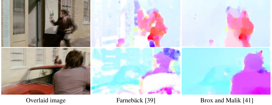
Figure 10: The left column shows the overlaid image of two consecutive frames. The middle and right columns are the visualization of two optical flow methods. Farnebäck [39] is able to capture the subtle motion patterns in the background, whereas LDOF [41] preserves motion boundaries more clearly.
