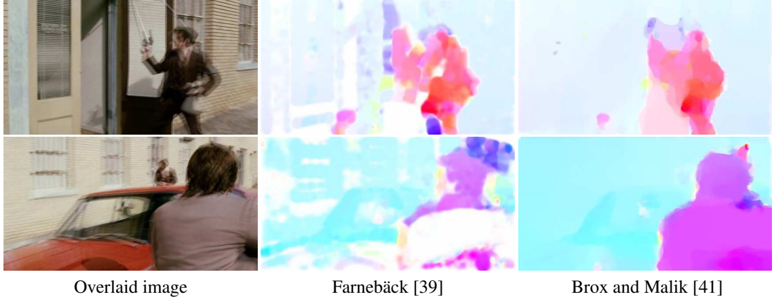
Figure 10: The left column shows the overlaid image of two consecutive frames. The middle and right columns are the visualization of two optical flow methods. Farneback [39] is able to capture the subtle motion patterns in the background, whereas LDOF [41] preserves motion boundaries more clearly.
