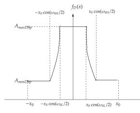
Figure 4: Object function for HPF of Figure 2, showing slight non linearity in the transition region.
