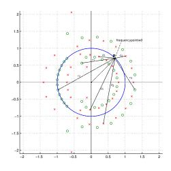
Figure 5: Calculation of transfer function from polezero plot at frequency  $\omega_0$ .
