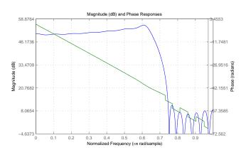
Figure 10: Magnitude and Phase Response after shifting poles at origin.
