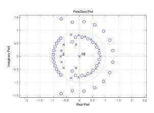
Figure 9: Pole-Zero Distribution after shifting poles at origin.
