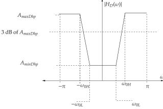
Figure 2: Desired high pass FIR filter characteristics to be used as denominator.
