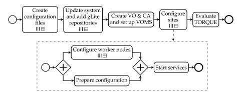
Figure 1: A workflow representation of *gLite experiment*. It consists of a workflow representing the whole process (top workflow) and a subprocess for the *Configure sites* phase (bottom workflow, executed for each site in parallel).
