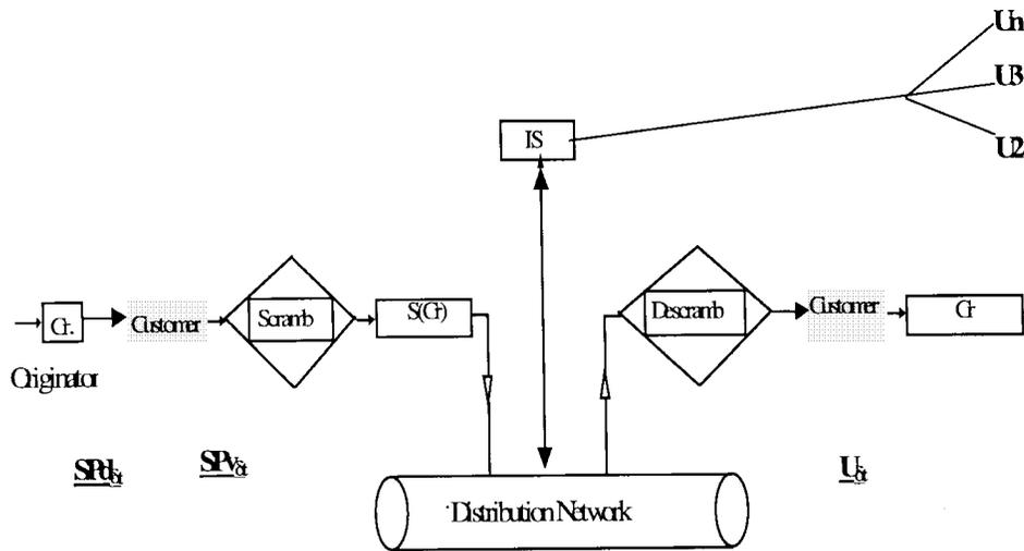
Fig. 5. Generic scheme for a distribution network.
