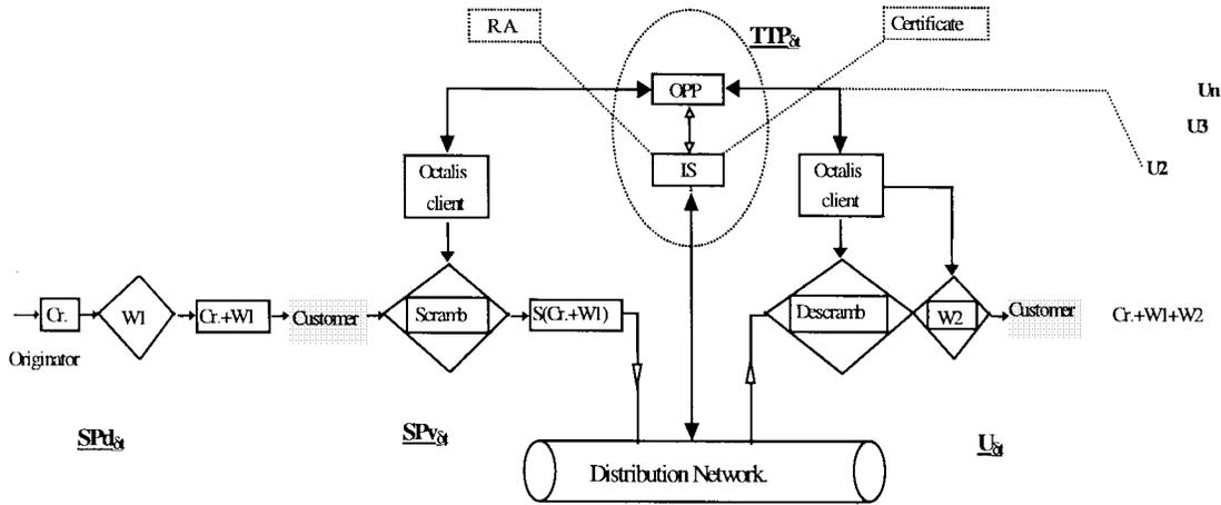
Fig. 7. IPR protection over the Eurovision network.
