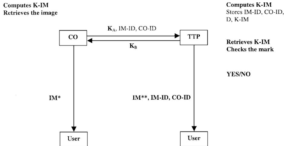
Fig. 4. The Diffie-Hellman protocol for watermarking (DHWM).
