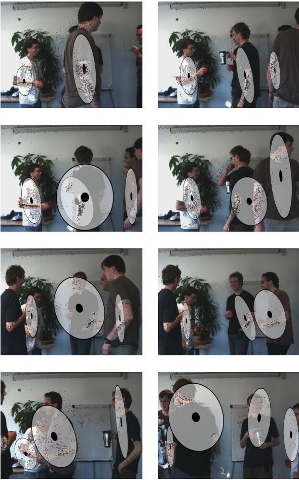
Fig. 7: A sample of the AV events detected in the CPP sequence of the RAVEL data set. The ellipses correspond to the localization of the events in the image plane. The method correctly detects and localizes 26 objects out of 33 (78.8%).
