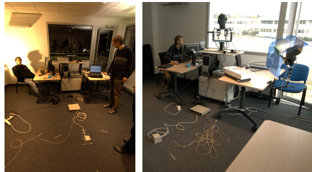
Fig. 3: Two views of the recording environment. The POP-EYE robot is in one side of the room. As shown, the sequences were shot with and without daylight providing for lighting variations. Whilst two diffuse lights were included in the setup to provide for good illumination, no devices were used to modify neither the illumination changes nor the sound characteristics of the room. Hence, the recordings are affected by all kind of audio and visual interferences and artifacts present in natural indoor scenes.
