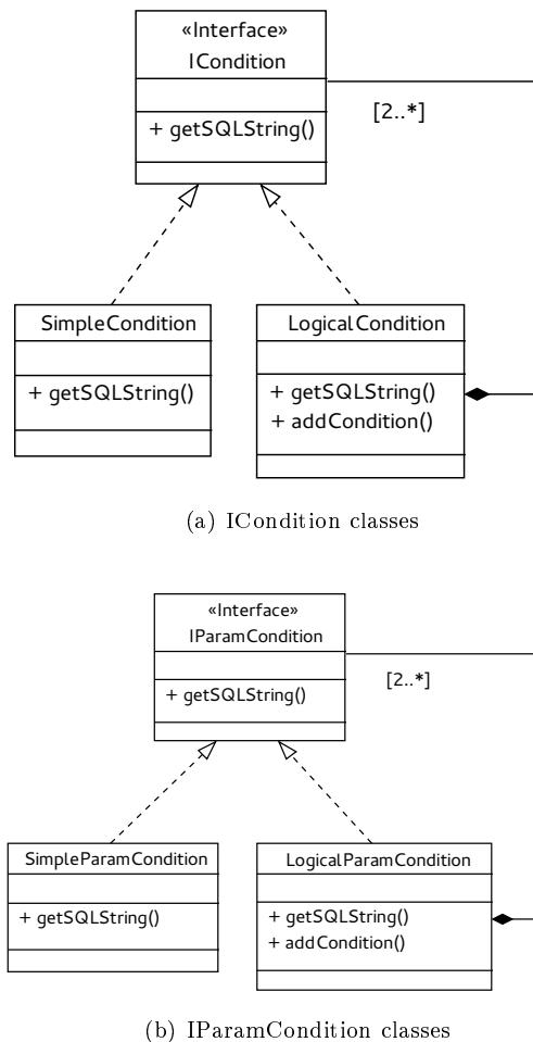
FIG. 15 – Condition-classes UML diagrams
