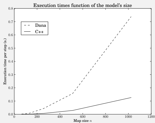
Figure 7: Execution time comparison between a DANA and C++ implementation for the Gray-Scott reaction diffusion model. The time to execute a single step is averaged over 1000 steps.
