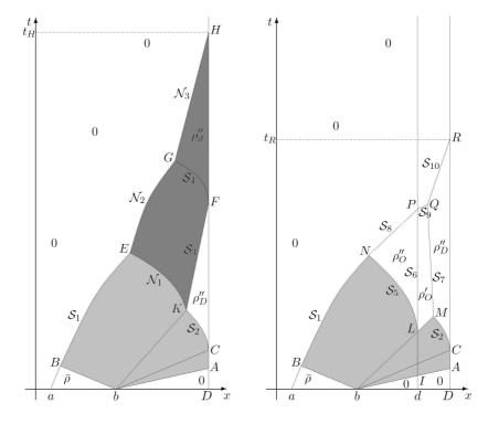
Figure 4: Wave-front tracking applied to (5.1)-(5.2). Left, the structure of the solution without obstacle  $(q \ge \max(f(\rho)))$ : the evacuation time is  $t_H$ . Right, in the presence of the obstacle, the evacuation time is  $t_R < t_H$ . (Taken from [10, 13].)
