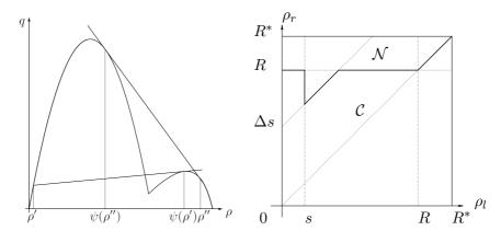
Figure 2: Left, the functions  $\psi$  and  $\varphi$ : their geometrical meaning. Right, the Riemann Solver: in C, the solution consists of classical waves only; in  $\mathcal{N}$ , also nonclassical shocks are present.
