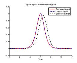
Fig. 2. The discrete signal  $y^d$ , the signal  ${}_fy^\varpi$  filtered by Butterworth filter, and the estimate  $y^\varpi_h$  obtained by the SCSA method with h=0.4.
