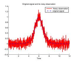
Fig. 1. The discrete signal  $y^d$  and the discrete noisy signal  $y^\varpi$  with  $SNR=11 \mathrm{dB}$ .
