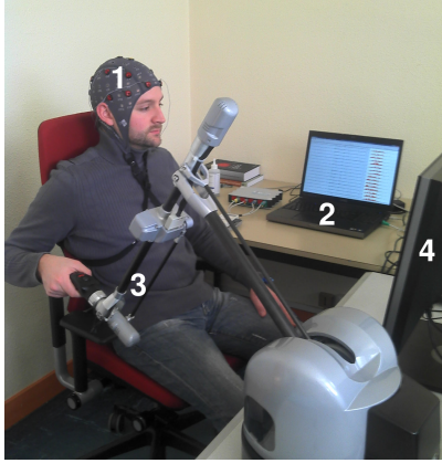
(a) Apparatus 1: EEG headset, 2: EEG acquisition, 3: haptic device, 4: LCD screen where the virtual scene is displayed.
