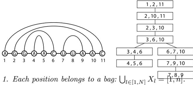
**Fig. 2.** An arc-annotated sequence and an associated tree decomposition. Each bag contains three positions, so the tree width of this tree decomposition is 2. As there is only one bag which does not respect the smooth property (the one with two children), the tree decomposition is 1-weakly-smooth.
