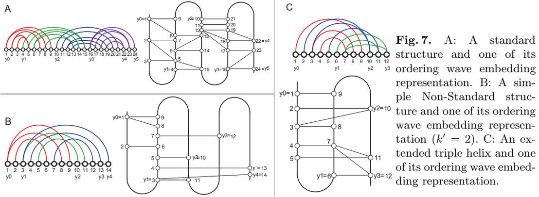
**Fig. 7.** A: A standard structure and one of its ordering wave embedding representation. B: A simple Non-Standard structure and one of its ordering wave embedding representation ( $k' = 2$ ). C: An extended triple helix and one of its ordering wave embedding representation.
