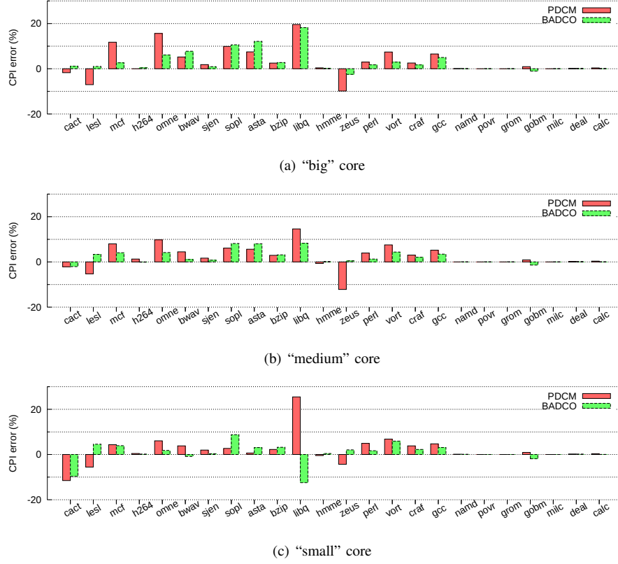
Figure 4. CPI error of PDCM and BADCO for the “small”, “medium” and “big” cores, with the uncore configuration “001”.
