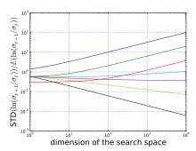
Fig. 2: Standard deviation of  $\ln(\sigma_{t+1}/\sigma_t)$  relatively to its expectation. Here  $\lambda=8$ . The curves were plotted using Eq. (21) and Eq. (22). On the left, curves for (right to left) n=2, 20, 200 and 2000. On the right, different curves for (top to bottom) c=1, 0.5, 0.2,  $1/(1+n^{1/4})$ ,  $1/(1+n^{1/3})$ ,  $1/(1+n^{1/2})$  and 1/(1+n).
