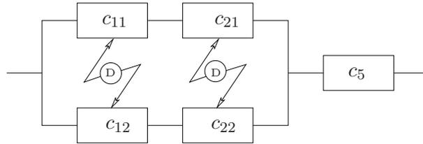
Figure 10: Series/parallel reliability block diagram of the example
