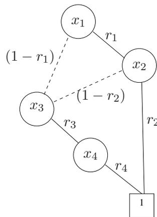
Figure 8: Positive ROBDD of the example for the order  $x_1 < x_2 < x_3 < x_4$ , with elementary reliabilities labelling the edges.
