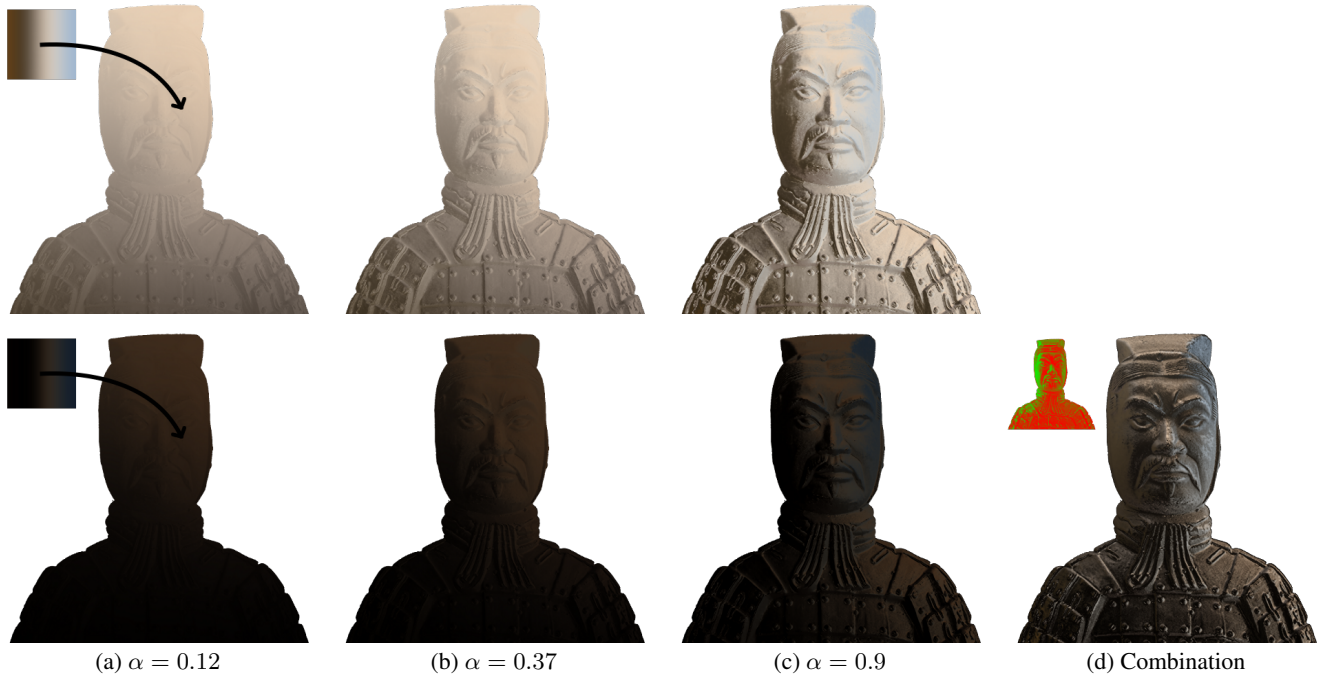
Figure 2: RGBN image. This result is obtained using a single gradient image as input and one anchor point. In the top row (a,b,c), the gradient is distorted (by increasing \alpha ) until the shape appears to have a 'diffuse-like' material. The same operation is done in the second row (a,b,c), except that the intensity of the input image was decreased. The final result (d) combines the images obtained in (c) using the Fresnel coefficient. All these operations are done in a single node in our system.
