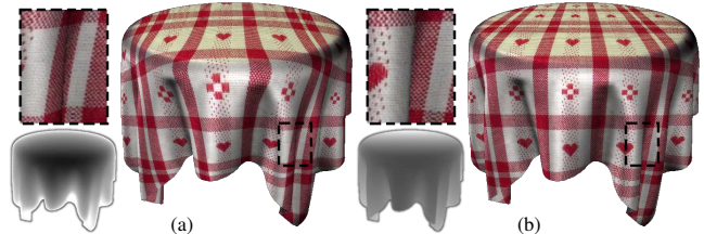
Figure 11: Texture mapping: compared to [Winnemöller et al. 2009] (a), our approach (b) better conveys discontinuities at occluding contours and produces more plausible deformations.
