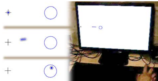
Figure 2. The stimuli displayed during one trial. Left top: the cursor begins at the starting position (cross hair) at the left. Left middle and right: the cursor midway between the starting position and the circular target at the right. The cursor is displayed as multiple alpha-blended copies, simulating a motion blur, to compensate for the screen’s refresh rate being lower than the mouse’s reporting rate. Left bottom: The cursor inside the target.
