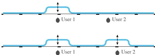
**Figure 8: (top) locally-bounded transformations allow User 1 to look behind bezels without disturbing User 2. (bottom) User 1 and User 2 can invoke the technique independently.**
