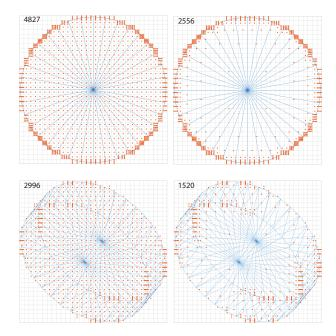
**Figure 6:** Ray distribution for sampling a cylinder. The red points denote rays which are perpendicular with the paper. The total number of rays along three orthogonal directions is given on top left of each figure. Left: uniform grid with local refinement. Right: multi resolution coarsening is used. Top: worst sampling directions. Bottom: optimized directions.
