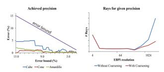
Figure 9: Precision and ray number tests. Left: Achieved vs. desired precision of volume for three different polyhedra. Right: The number of rays used to obtain a given precision, depending on the EBPI resolution, with coarsening (red) or without (blue).
