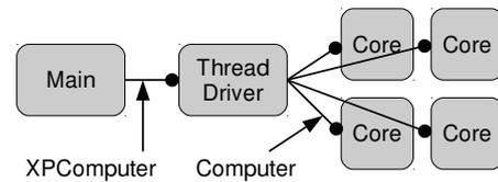
Figure 2: Application architecture with four threads of computation running in parallel for a shared memory machine. Each instance of the **Core** component runs in a distinct thread created by the **ThreadDriver** component.
