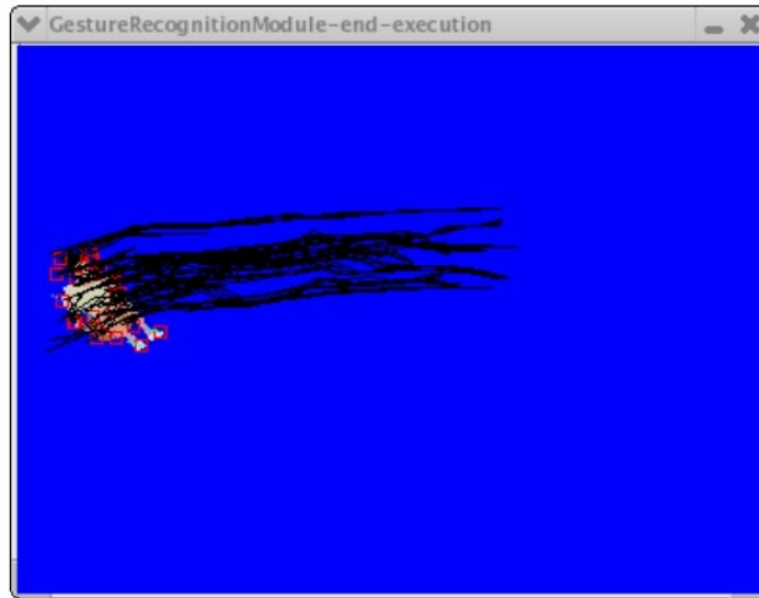
Figure 2: Synthetic data-set: Red rectangles represent the tracked descriptors and the lines represent their trajectories.
