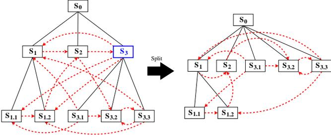
Figure 4: Split operator in MILES algorithm. The blue box represents the state to be split. Red dashed lines represent events. Notice that the split operator suppresses the state  $S_3$  and its arriving and leaving events, and ascends the children of  $S_3$  in the hierarchy.
