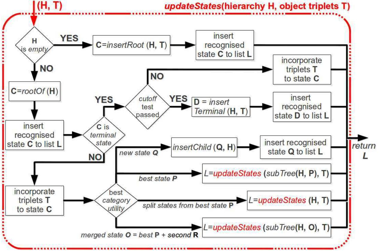
Figure 3: Scheme of the state concept updating algorithm.
