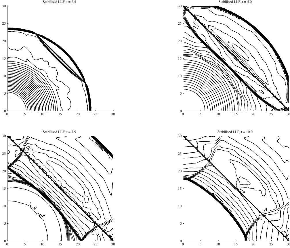
Figure 18: Circular dam break over discontinuous bed using a locally refined mesh. 30 free-surface contours for the LLFs scheme taken from [?].
