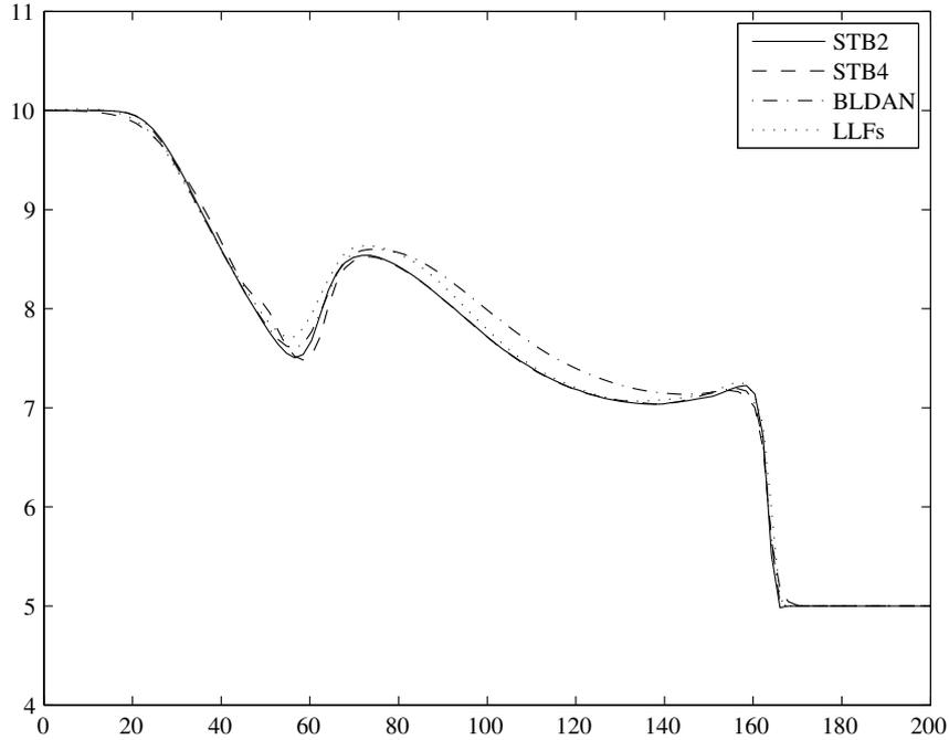
Figure 16: Partial dam break. Slice plots of water height at final time  $t = 7.2$  along the line  $y = 135$  for the blended non-space-time scheme, for the LLFs scheme and for the discontinuous STB scheme with  $CFL = 2, 4$ .
