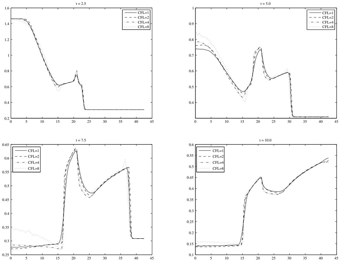
Figure 13: Plots of the free surface along the line  $x = y$ . The slices are taken at  $t = 2.5$ ,  $t = 5.0$ ,  $t = 7.5$  and  $t = 10.0$ . In each figure the results for  $\text{CFL} = 1$ ,  $\text{CFL} = 2$ ,  $\text{CFL} = 4$  and  $\text{CFL} = 8$  are shown.
