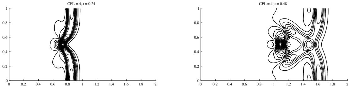
Figure 6: Perturbation to the lake at rest when solved with the discontinuous STB scheme with CFL = 4. 50 water-height contours between values 0.992 and 1.012 at  $t = 0.24$  (left) and  $t = 0.48$  (right) are plotted.
