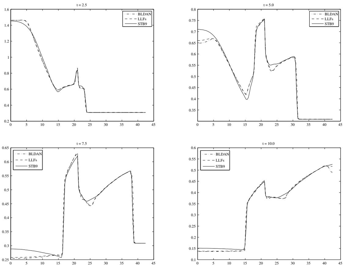
Figure 21: Circular dam break over discontinuous bed using a locally refined mesh. Plots of the free surface along the line  $x = y$ . The slices are taken at  $t = 2.5$ ,  $t = 5.0$ ,  $t = 7.5$  and  $t = 10.0$ . In each figure the results for the blended LDAN scheme, the LLFs scheme and the discontinuous STB scheme (CFL = 9) are shown.
