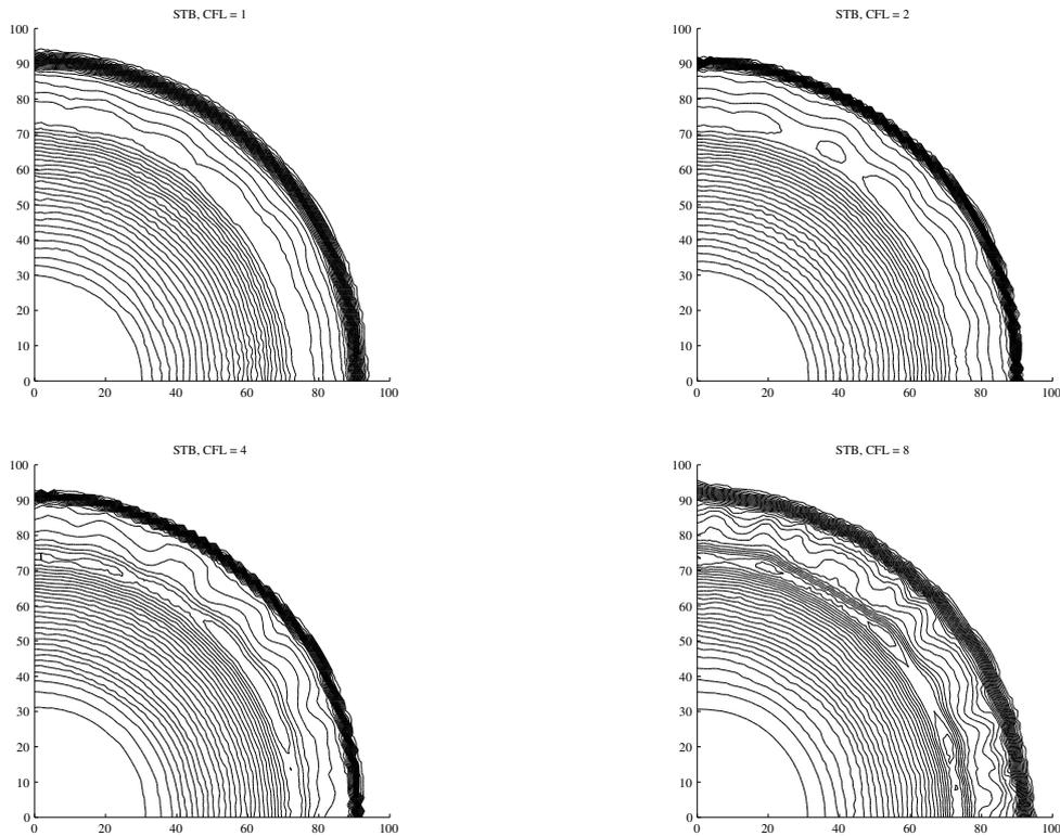
Figure 1: Circular dam break. 30 Froude-number contour plots of the discontinuous STB scheme for  $\text{CFL} = 1$  (top left),  $\text{CFL} = 2$  (top right),  $\text{CFL} = 4$  (bottom left) and  $\text{CFL} = 8$  (bottom right).
