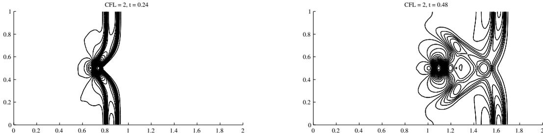
Figure 5: Perturbation to the lake at rest when solved with the discontinuous STB scheme with  $\text{CFL} = 2$ . 50 water-height contours between values 0.992 and 1.012 at  $t = 0.24$  (left) and  $t = 0.48$  (right) are plotted.
