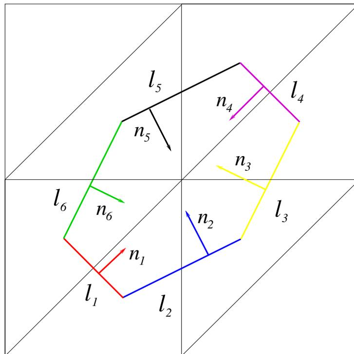
Figure 22: Sketch of the vertex-centred finite volume scheme
