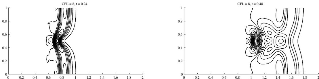
Figure 7: Perturbation to the lake at rest when solved with the discontinuous STB scheme with CFL = 8. 50 water-height contours between values 0.992 and 1.012 at  $t = 0.24$  (left) and  $t = 0.48$  (right) are plotted.
