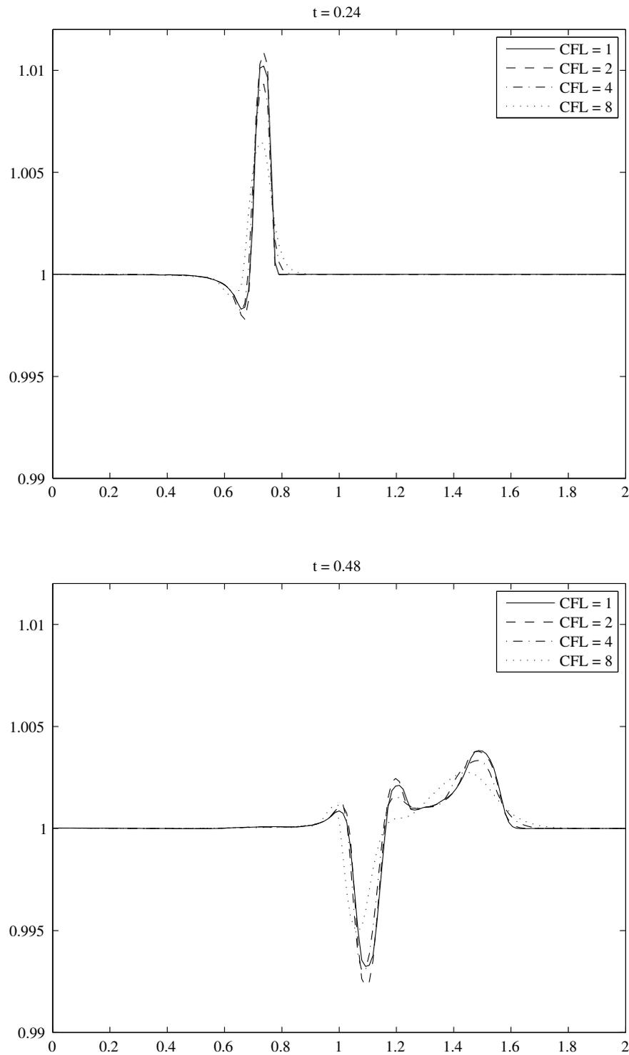
Figure 8: Perturbation to the lake at rest when solved with the discontinuous STB scheme with CFL = 1, CFL = 2, CFL = 4 and CFL = 8. Slice plots are shown along the line  $y = 0.5$  at  $t = 0.24$  and  $t = 0.48$ .
