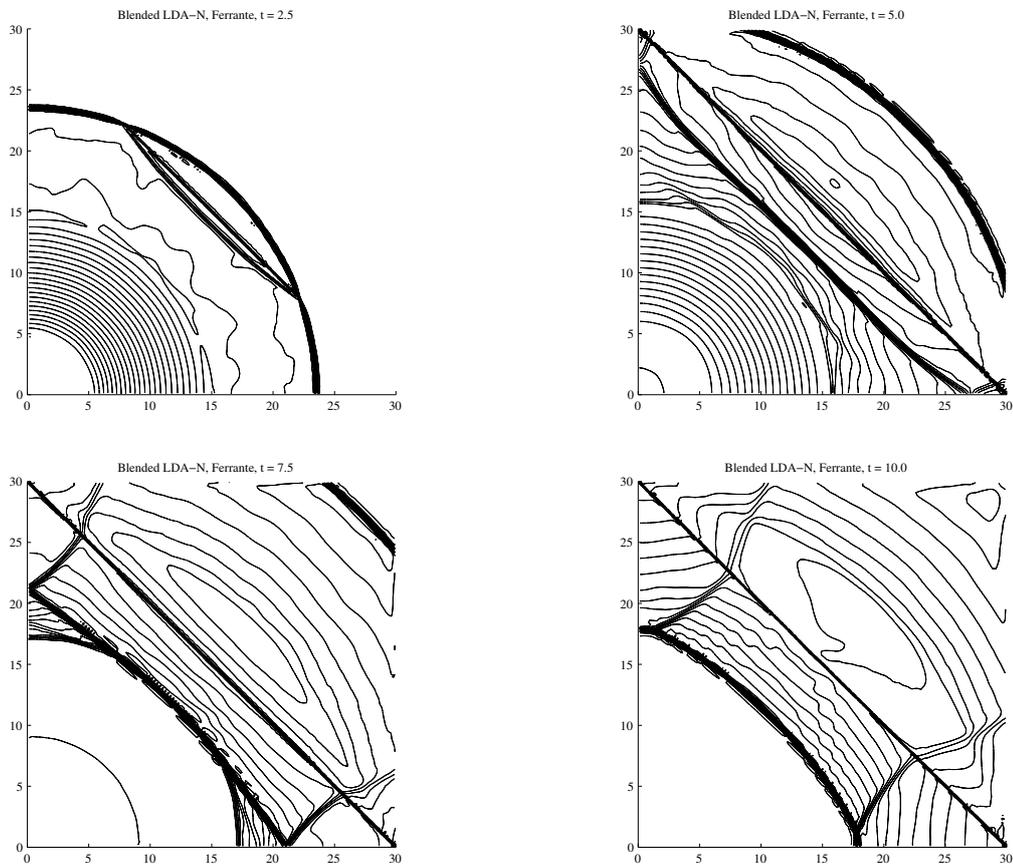
Figure 17: Circular dam break over discontinuous bed using a locally refined mesh. 30 free-surface contours for the blended scheme where the LDA part is computed as in [?].
