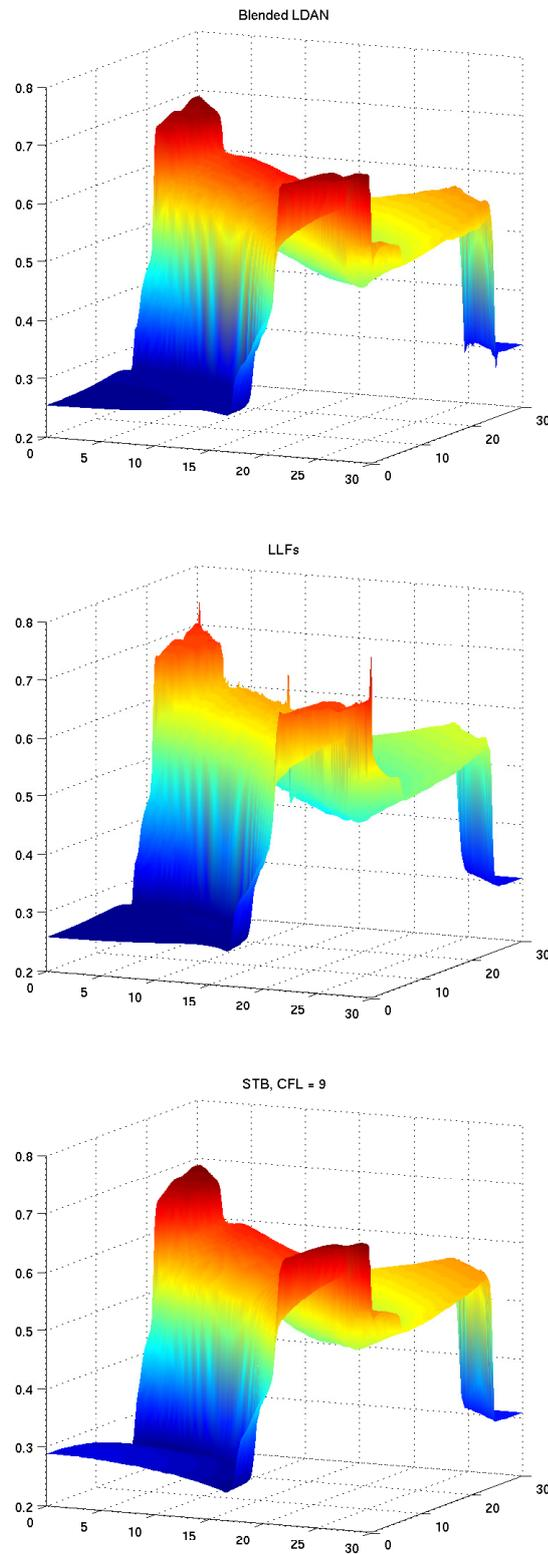
Figure 20: Circular dam break over discontinuous bed using a locally refined mesh. 3D free-surface plots at  $t = 7.5$  for the blended LDAN scheme, the LLFs scheme and the discontinuous STB scheme (CFL = 9).
