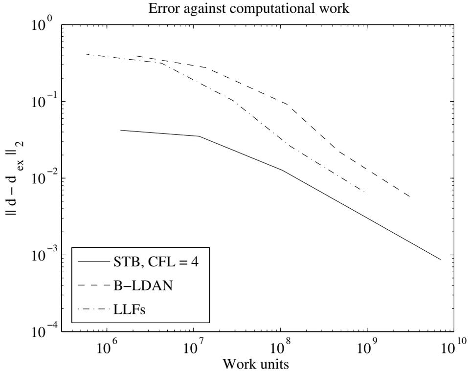
Figure 14: Travelling vortex. Computational work needed to achieve a given accuracy for the LLFs scheme, for the blended non-space-time scheme and for the discontinuous STB scheme with CFL = 4.
