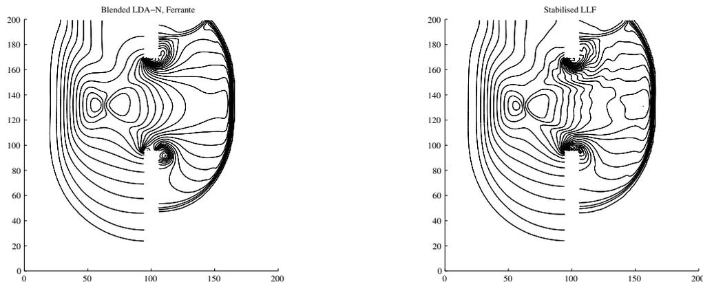
Figure 15: Partial dam break. 30 water-height contours between 4 and 9.95 for the blended scheme and the LLFs scheme at the end of the integration  $t = 7.2$ . This figure is directly comparable to Figure 10 for the space-time DRD scheme.
