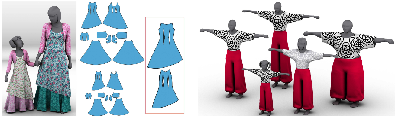
Figure 1: Design preserving garment transfer: (left) transfer of a multi-layer outfit from a woman to a young girl; automatically graded patterns (bottom) shown to scale. The zoomed-in source and target patterns for the back panel highlight the subtle changes in shape. (right) Dancer outfit transferred from the female in the center to a variety of other characters. ©Laurence Boissieux 2012
