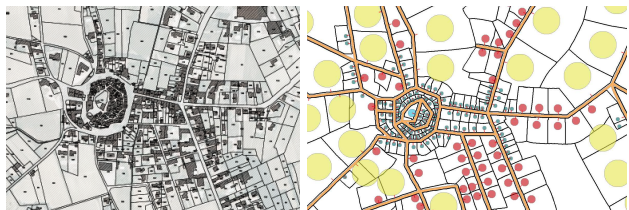
Fig. 12 Comparison of real versus generated land parcels on terrains with similar roads and building distributions.
