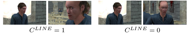
Figure 9: Line of action score. Top: In the left image, the gaze direction of the main actor defines the line of action. Bottom: the gaze direction changes because the camera has crossed the line, resulting in a poor cut. Bottom: keeping the line of action result in a smooth cut
