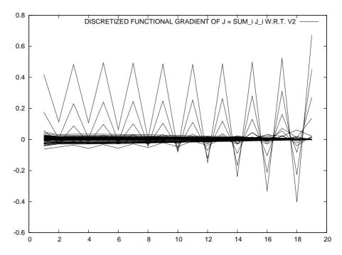
Figure 7: Quasi-Newton steepest descent - 200 iterations of  $\partial \mathsf{J}/\partial v_2$
