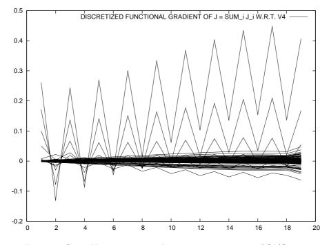
Figure 9: Quasi-Newton steepest descent - 200 iterations of  $\partial \mathsf{J}/\partial v_4$
